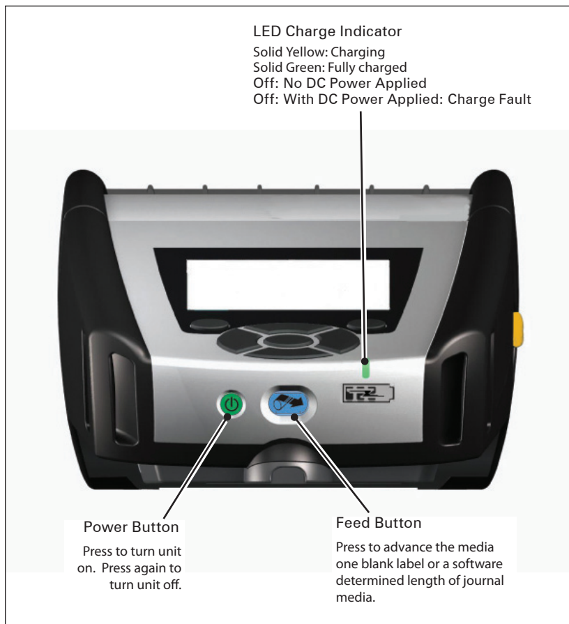
Figure 14: Standard Control Panel for QLn Series
